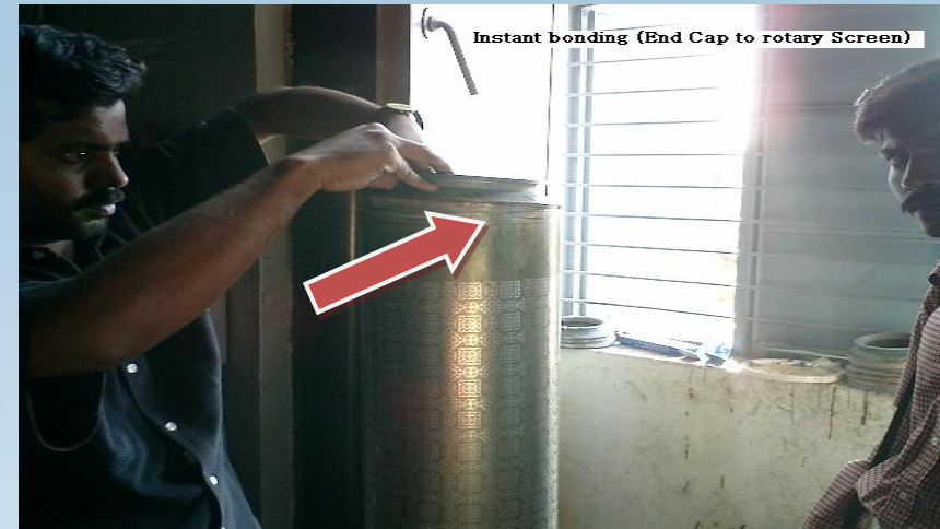
End cap to rotary screen Bonding
