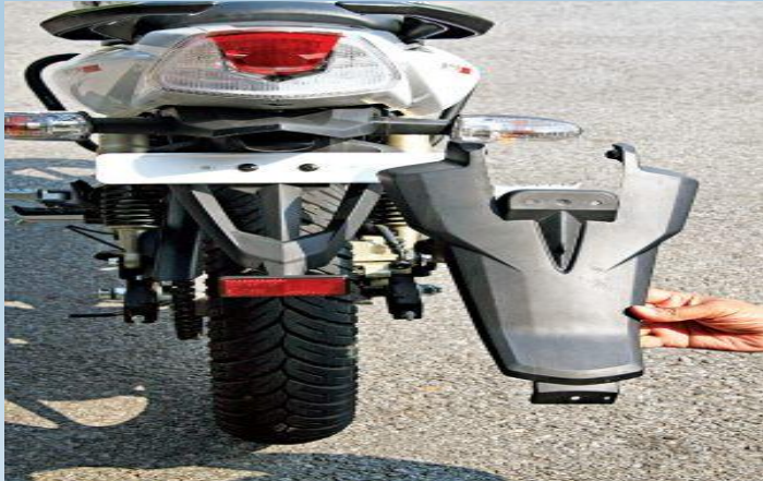
Repairing of mud guard
