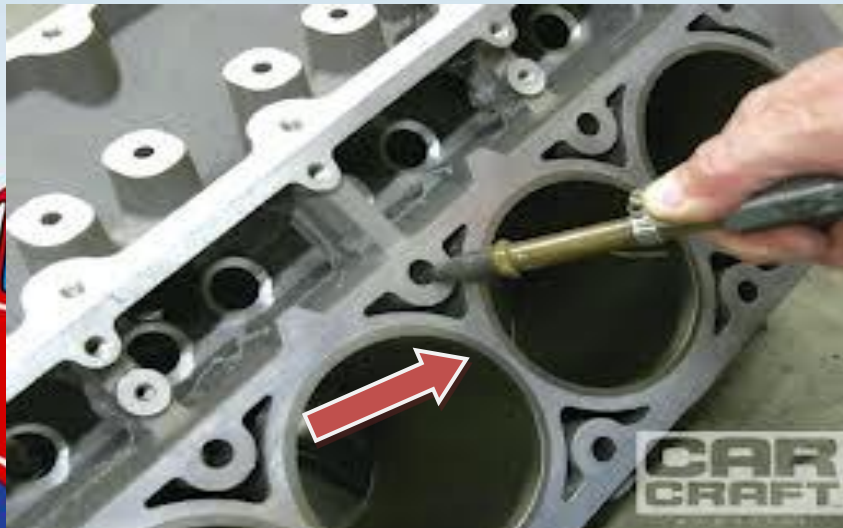
Sealing pasting in engine head repairing
