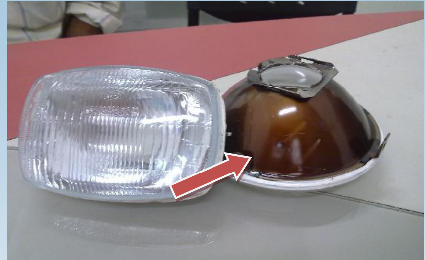
HEAD LIGHT BONDING WITH PIGMENT (REFLECTOR TO GLASS)
