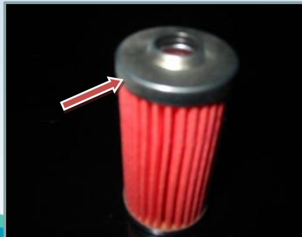
End cap to paper bonding in automobile filter
