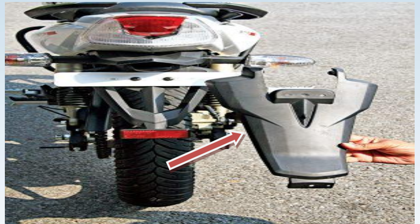
Repairing of mud guard
