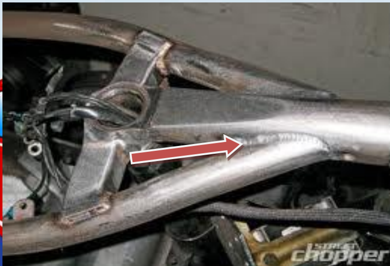
Smoothing of welded area
